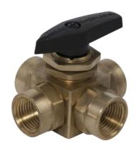
Kantleak<sup>™</sup> 4-Way Instrumentation Ball Valves are designed with double O-ring seal providing over 20,000 cycles without leakage and an exclusive stem seal that never needs tightening. Valves can be panel mounted for instrumentation applications. Applications include refrigerant service, oxygen and vacuum service. Porting options are available
