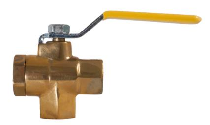
Kantleak™ Ball Valves are designed with double o-ring protection and our exclusive stem seal never needs tightening. Our valves also feature forged brass CDA 377, chrome plated brass ball, blow-out proof stem, and easy turn handle.
