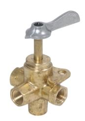
The 100 Series non-lubricated selector valves are designed to operate in systems where instantaneous port selection is desired. Since lubricants are not used, re-lubrication is not required. There is no lubricant to freeze and lock the valve or to contaminate fine fluids. The O-ring sealed cap and stem eliminate leakage. The series is designed for panel or bracket mounting. Standard with pointer lever to indicate the desired porting selection and can be rotated 360 degrees.
