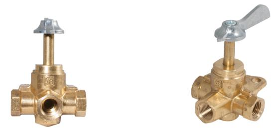
210 Series non-lubricated selector valves are designed to operate in systems where instantaneous port selection is desired. Since lubricants are not used, re lubrication is not required. There is no lubricant to freeze and lock the valve or to contaminate fine fluids. The O ring sealed cap and stem eliminate leakage. The series is designed for panel or bracket mounting Standard with pointer lever to indicate the desired porting selection and can be rotated 360
