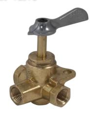
The 110 Series non-lubricated selector valves are designed to operate in systems where instantaneous port selection is desired. Since lubricants are not used, re-lubrication is not required. There is no lubricant to freeze and lock the valve or to contaminate fine fluids. The O-ring sealed cap and stem eliminate leakage. The series is designed for panel or bracket mounting. Standard with pointer lever to indicate the desired porting selection and can be rotated 360 degrees.
