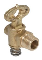
**Instantaneous** off-on operation with 360° rotation. The lapped brass body and plug are individually mated, providing an excellent quality, low friction valve. Valves are extensively used for water process piping and air supply systems.
