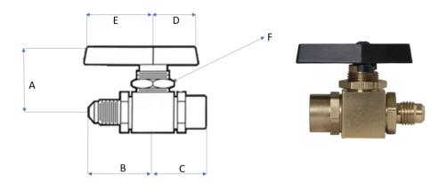
Kantleak™ Instrumentation Ball Valves are designed double o-ring stem seals to provide over 20,000 leak free cycles. These valves also feature an exclusive stem seal design that never needs tightening and can be panel mounted for instrumentation applications.
