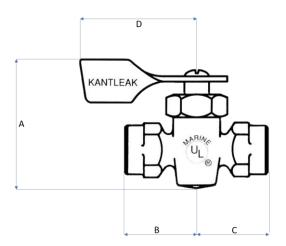
The Kantleak™ Marine Fuel Shut Off Valve is AP approved for use on motor craft fuel lines and is standard with pointer lever and an internal 90° turn stop mechanism to assure positive location of the on and off position. Corrosion proof internal construction assures maximum salt atmosphere protection.
