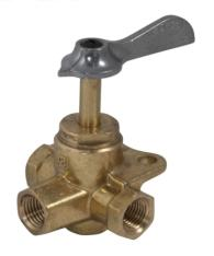
The 210 Series non-lubricated selector valves are designed to operate in systems where instantaneous port selection is desired. Since lubricants are not used, re-lubrication is not required. There is no lubricant to freeze and lock the valve or to contaminate fine fluids. The O-ring sealed cap and stem eliminate leakage. The series is designed for panel or bracket mounting. Standard with pointer lever to indicate the desired porting selection and can be rotated 360 degrees.
