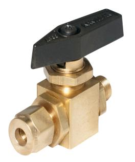
Kantleak<sup>™</sup> Instrumentation Ball Valves are designed with double o-ring stem seals to provide over 20,000 leak free cycles. These valves also feature an exclusive stem seal design that never needs tightening and can be panel mounted for instrumentation applications.
