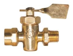
The Kantleak<sup>™</sup> Marine Fuel Shut Off Valve is AP approved for use on motor craft fuel lines and is standard with pointer lever and an internal 90° turn stop mechanism to assure positive location of the on and off position. Corrosion proof internal construction assures maximum salt atmosphere protection.
