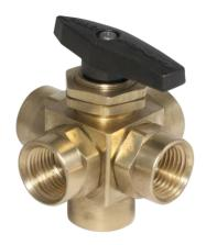
Kantleak<sup>™</sup> 5-Way Instrumentation Ball Valves are designed with double O-ring seal providing over 20,000 cycles without leakage and an exclusive stem seal that never needs tightening. Valves can be panel mounted for instrumentation applications. Applications include refrigerant service, oxygen and vacuum service. Porting options are available
