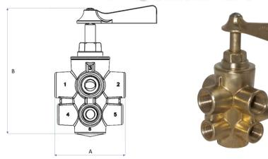
The Six Port Selector Valves are designed for engine applications where a fuel return or spill back is required. The closed bottom with O-ring sealed cap and stem eliminates external leakage. These valves are widely used in the trucking and marine industry, along with manufactures of diesel generating plants. The specially formulated high temperature, low friction grease permits sealing and ease of turning from -40° to 180° F at a maximum operating pressure of 15 P.S.I.
