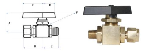
Kantleak<sup>™</sup> Instrumentation Ball Valves are designed with double o-ring stem seals to provide over 20,000 leak free cycles. These valves also feature an exclusive stem seal design that never needs tightening and can be panel mounted for instrumentation applications
