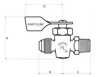
The Kantleak<sup>™</sup> Marine Fuel Shut Off Valve is AP approved for use on motor craft fuel lines and is standard with pointer lever and an internal 90° turn stop mechanism to assure positive location of the on and off position. Corrosion proof internal construction assures maximum salt atmosphere protection.
